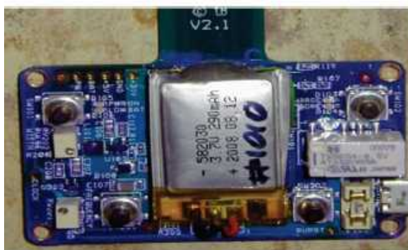
Figure 2: Bottom of the PoNS™ Neuro-stimulator board
